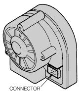
The arm/disarm output signal from the GM (STDWA) is provided to the Tilt sensor, FIS sensor and the siren simultaneously. The arm/disarm signal is a switched ground that signals the components of DWA armed/disarmed status.
